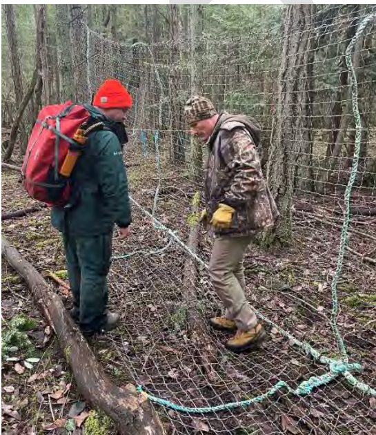
Figure 8. Aquaculture Netting as Installed During the Parks Canada Fencing Trials (Tooby et al., 2022)
